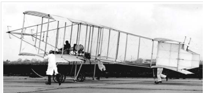
Figure 4: Replica 1911 Bristol Boxkite, built by Miles Aircraft Ltd for the film “Those Magnificent Men in their Flying Machines” using authentic materials, which included Ash for the undercarriage skids. 6 May 1964, pilot George Miles FRAeS. Photo courtesy Karen Miles.
