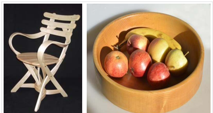
Figure 3: Coppiced Ash split from an ancient stool in Bradfield Woods and bent to form this chair, made by a local craftsman Dan Hussey, who kindly donated this photograph. Ash turns well.
