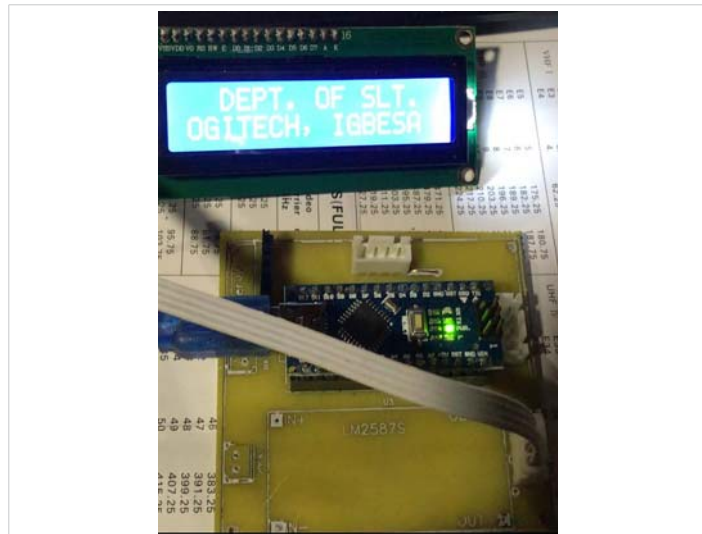
Figure 8: Liquid Crystal Display is Connected with Arduino Nano Board for Uploading.
