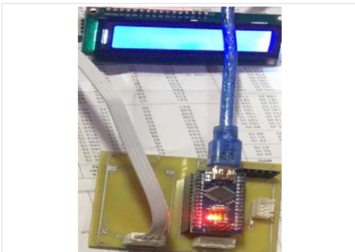
Figure 6: J-S-T connected to LCD from PCB.
