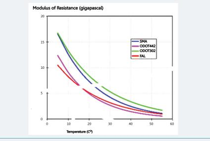
Figure 2: The relationship between temperature and modulus of variation for different materials.
