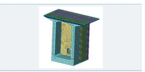
Figure 4: Zero block finite element model. Blue and cyan unit are box girder of zero block, yellow and pink unit are diaphragm plate of zero block.
