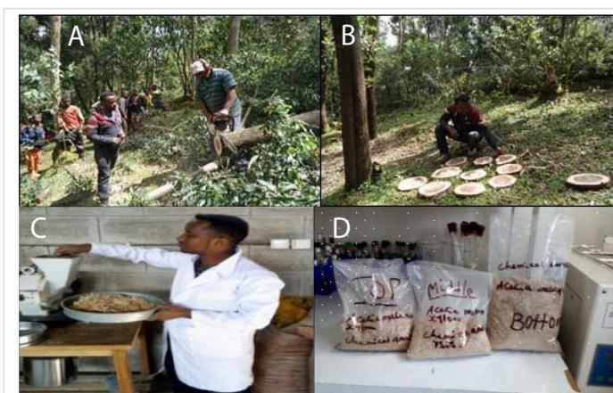
Figure 2: Sample collection and preparation: cutting disks and coding (A&B), Grinding (C&D).
