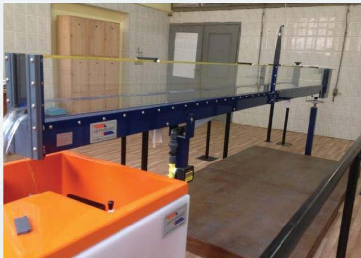
**Figure 1:** Open channel Armfield flume Model No. C4-MKII-5.0-11 with a basic hydraulic bench Model No. F1-10-A.
